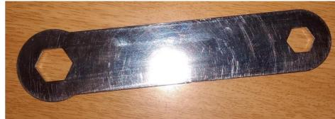
NB: In the kit there are two spanners that look like the above image. Keep these in you vehicle. These are to remove the front styling bar if you need to gain access to the tow eye.
