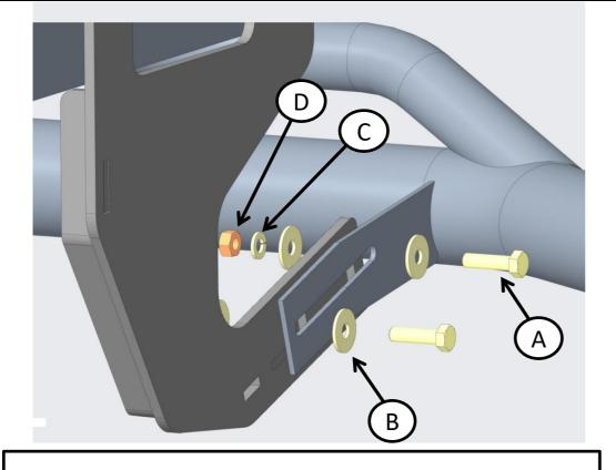
The mounting bracket has three slots. Use the rear two slots for vehicle models 2018 and below. Use the front two slots for models 2019 and up.
