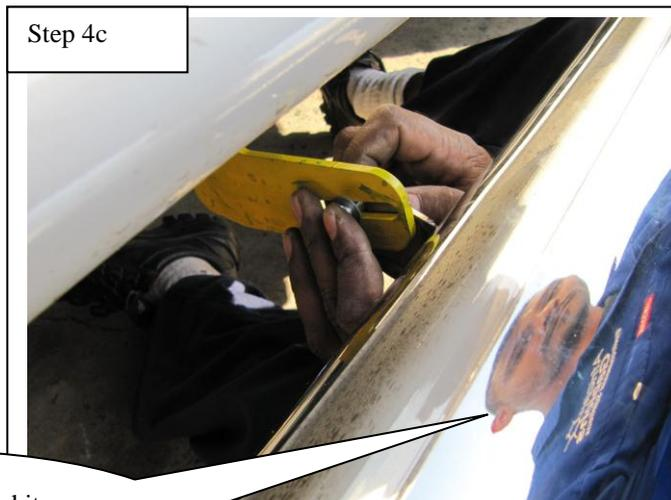
Using the bolts from the kit provided, secure the side step. Align and tighten the bar.
