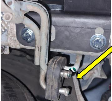
Drop the exhaust by unclipping the rubber mounting, this will make room to have the Towbar put into place.
